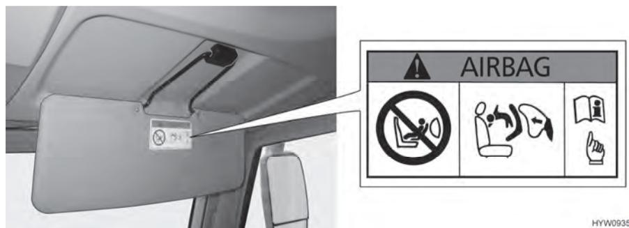
Fig. 13 Warning notice on child restraint system (front passenger's seat sun visor)
