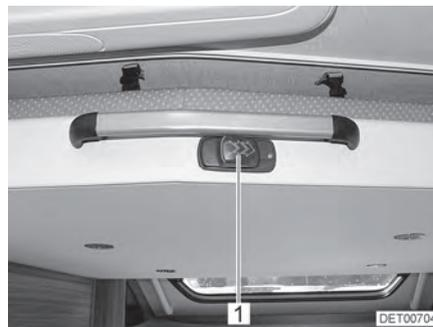
Fig. 75 Pull-down bed with lock
