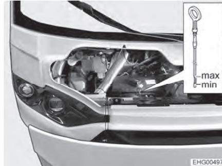
Fig. 12 Oil dipstick (engine oil)
