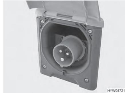
Fig. 103 230 V connection on the vehicle (CEE socket outlet)
