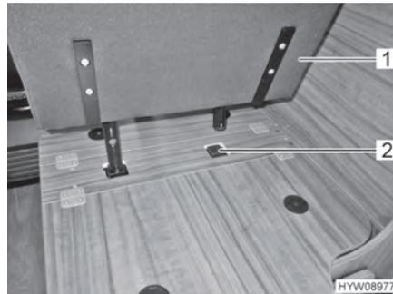
Fig. 19 Place the attachable seat in the holder
