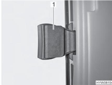
Fig. 37 Sliding window without lock
