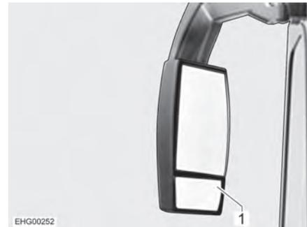
Fig. 28 Retrovisor exterior (modelo I)
