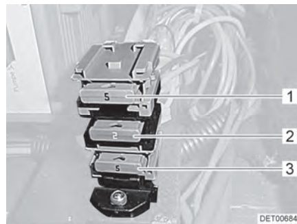
Fig. 104 Fuses next to the transformer/rectifier
