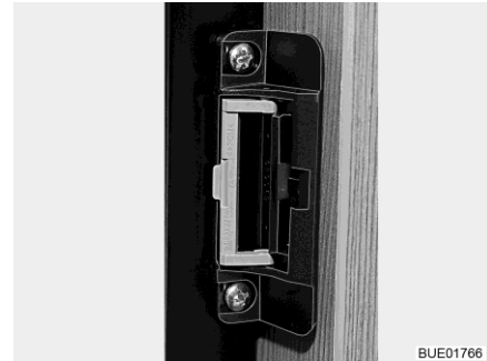
Fig. 98 Locking device in ventilation position
