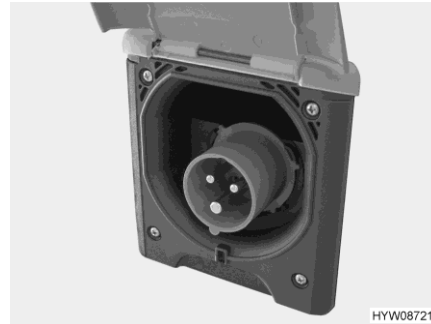
Fig. 75 230 V connection on the vehicle (CEE socket outlet)
