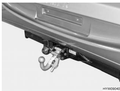
Fig. 9 Caravan coupling, detachable (example illustration)
