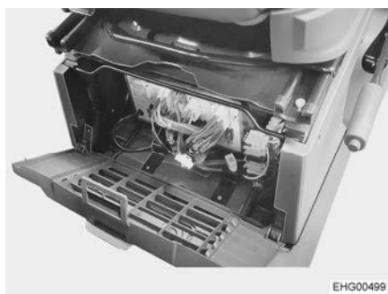
Fig. 151 Position of transformer/rectifier (Stellantis), illustration similar
