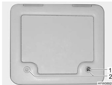
Fig. 210 Flap for the sewage tank
