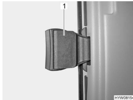
Fig. 58 Sliding window without lock
