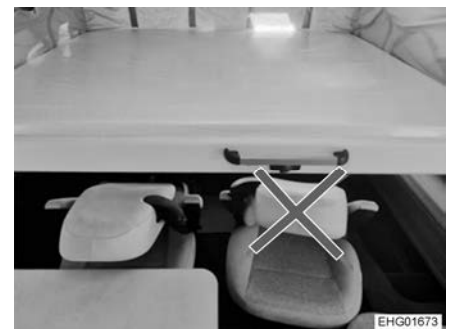
Fig. 103 Seats incorrectly adjusted
