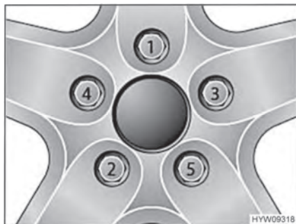
Fig. 94 Tightening the wheel nuts or wheel bolts cross-wise
