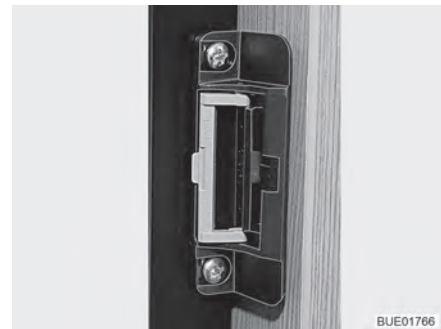
Fig. 74 Locking device in ventilation position
