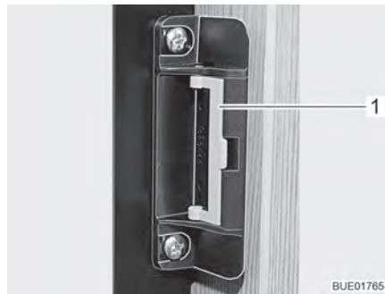
Fig. 73 Locking device in normal position
