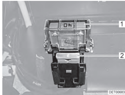
Fig. 60 Fuses on the living area battery
