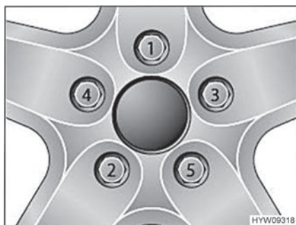
Fig. 88 Tightening the wheel nuts or wheel bolts cross-wise
