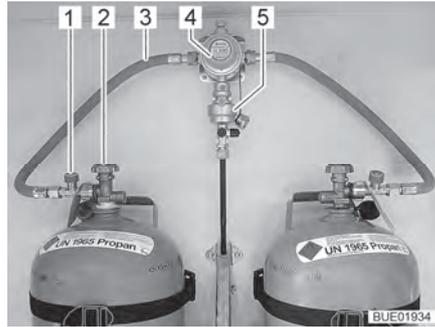
Fig. 67 Gas bottles with DuoControl
