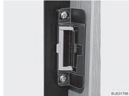
Fig. 102 Locking device in ventilation position
