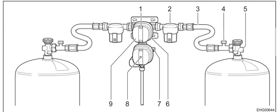
Fig. 69 Gas pressure regulating system DuoControl CS
