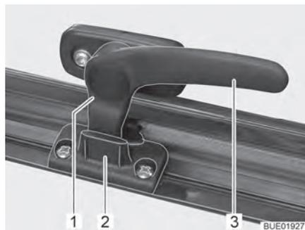
Fig. 20 Catch lever in "continuous ventilation" position
