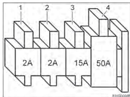
Fig. 83 Fuses on the starter battery
