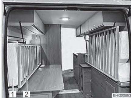
Fig. 46 Mattresses and bed bases transport position
