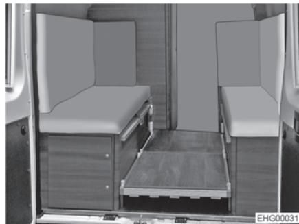
Fig. 51 Bunk bed, converted into seating group
