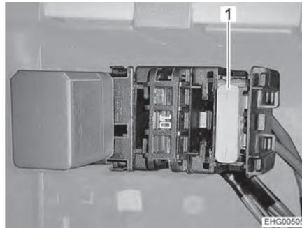
Fig. 87 Fuse on B column, right-hand side of vehicle
