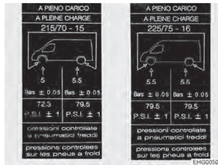
Fig. 129 Tyre pressure information sticker on B column (example)
