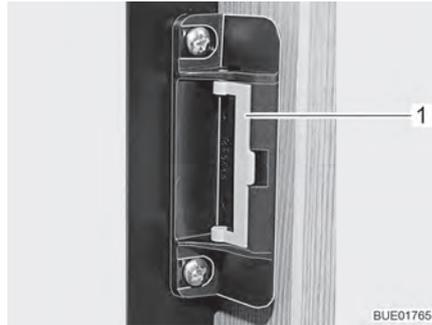
Fig. 101 Locking device in normal position
