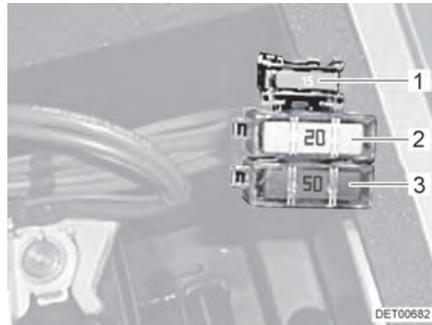
Fig. 81 Fuses on the starter battery without charging booster
