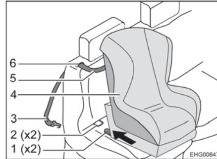
Fig. 15 Fastening with top tether
