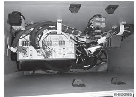
Fig. 75 Transformer/rectifier position (Ford)
