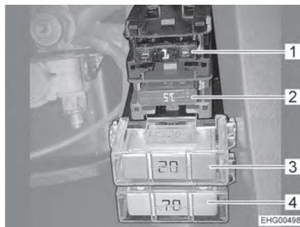
Fig. 82 Fuses on the starter battery with charging booster
