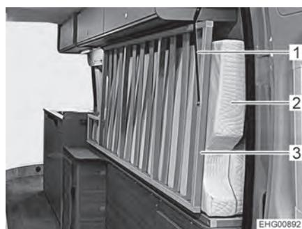
Fig. 45 Right-hand bed in transport position
