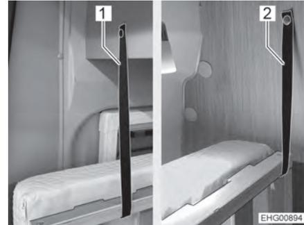
Fig. 47 Retaining straps for left-hand bed
