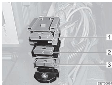
Fig. 87 Fuses next to the transformer/rectifier
