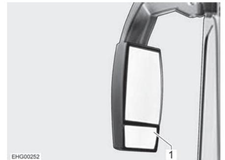
Fig. 20 Retrovisor exterior (modelo I)
