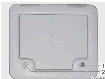
Fig. 155 Flap for the sewage tank
