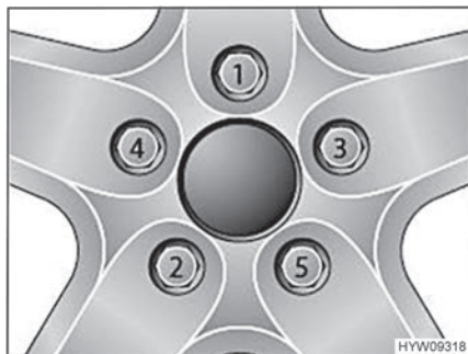
Fig. 88 Tightening the wheel nuts or wheel bolts cross-wise
