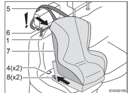
Fig. 8 Fixing with Isofix
